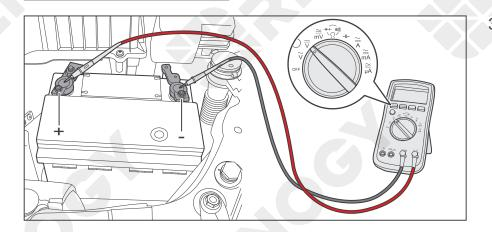
3. Read the voltage of the main vehicle battery.
