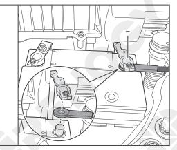
1. Attach the ring terminal of the negative Battery Adapter Cable (input) to the negative bolt of the starter battery.
