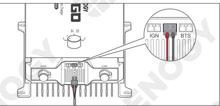
Insert the voltage sensor terminal block to the BVS port.
