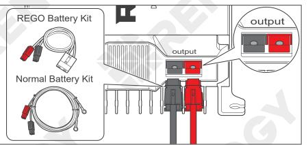
1. For the Output terminal, align the Battery Adapter Cable's Anderson PP75 connectors to the correct orientation and polarity.
