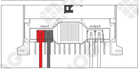
6. Insert the Anderson PP75 connectors into the Input terminal.
