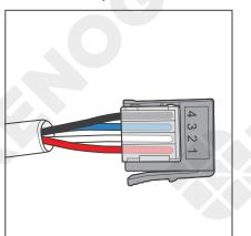
Insert the bare wires of the Drop Cables (sold separately) all the way into the wire ports of the Drop Plugs (not included) following the Drop Plug pinout. The red PS+ wire goes to pin 1, the white CAN\_H wire goes to pin 2, the blue CAN\_L wire goes to pin 3, and the black PSwire goes to pin 4.
