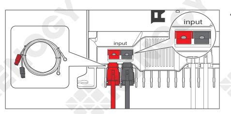
4. For the Input terminal, align the Battery Adapter Cable's Anderson PP75 connectors to the correct orientation and polarity.
