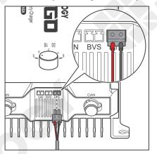
1. Insert the temperature sensor terminal block into the BTS port of the battery charger.
