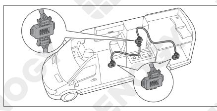
3. Locate the drop tap (not included) on the RV-C bus that is the closest to the installation site of the battery charger. The drop taps are usually located above the entry door, in the bathroom, or under the bed in the RV.
