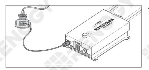
Connect either of the CAN Communication Ports of the battery charger and other REGO devices to the drop sockets on the drop tap with the Drop Cables.
