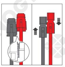
2. Bind the Anderson PP75 connectors by sliding the side grooves.
