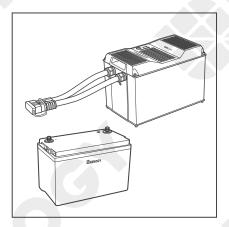
1. Inspect the auxiliary battery for any visible damage including cracks, dents, deformation, and other visible abnormalities. All connector contacts shall be clean, dry, and free of dirt and corrosion.
