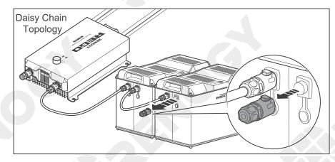
1. Remove the Terminator Plug from the REGO device at either end of the daisy chain.
