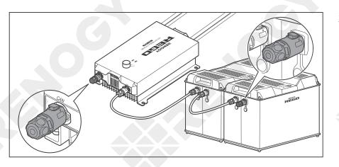
2. Plug the Termionator Plugs (sold separately) into the vacant CAN **Communication Ports** on the first and last **REGO** devices.
