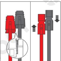
5. Bind the Anderson PP75 connectors by sliding the side grooves.
