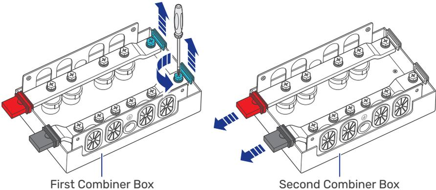
**Step 2:** Align the busbar ports.
