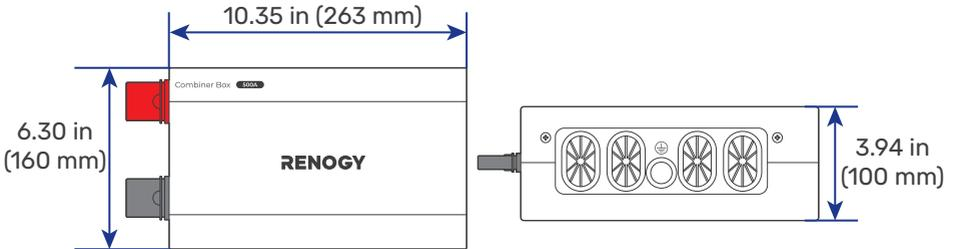
**i** Dimension tolerance:  $\pm 0.2$  in (0.5 mm)
