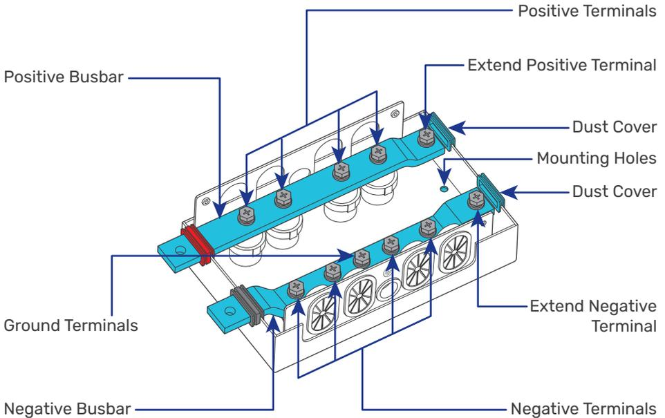
**i** Each busbar terminal is equipped with a terminal bolt, a spring washer, and a flat washer.
