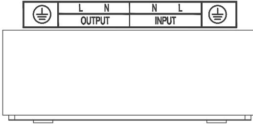
2.Make note of the AC output terminals from left to right (Ground, Live, Neutral) and the AC Input terminals from left to right (Neutral, Live, Ground).
