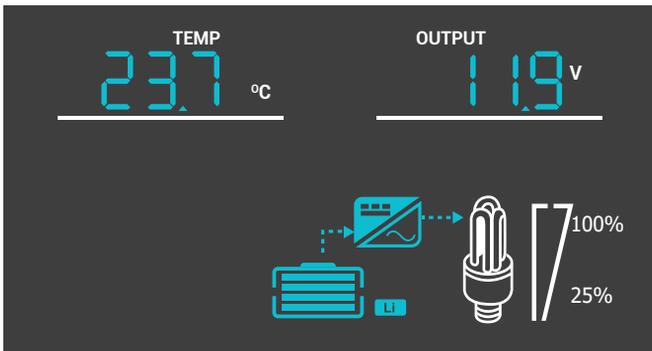
Inverter Temperature Celsius / Output Volts AC
