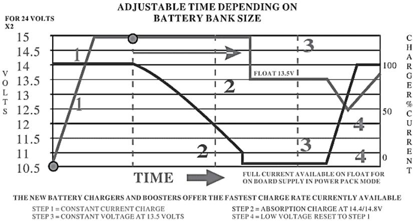
**Bulk Stage:** The charger will supply constant current until the battery voltage reaches the boost voltage. The software will calculate the time charging began up until the battery voltage reaches 0.3V below the boost voltage. It uses this time to as  $T_0$  and  $T_0 \times 10 = T_1$ .
